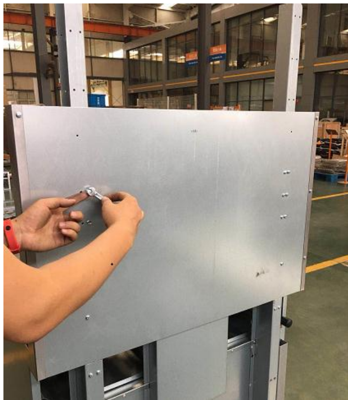
3. Lift Cheese melter and attach it to the proper position of the support column
